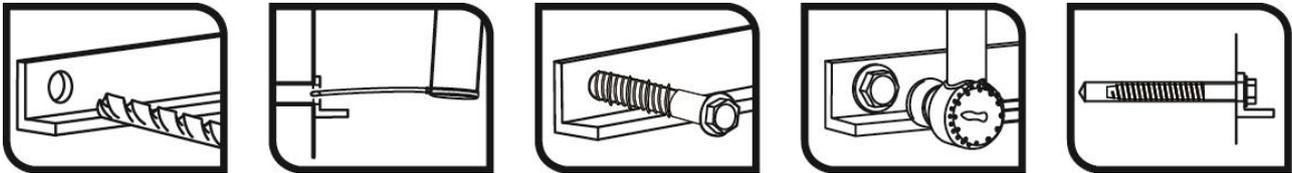
Anchor shall be installed using a torque wrench or an electrical impact driver; power input: 500 W; torque: 50-250 Nm. (e.g: Bosch GDS 18E)
